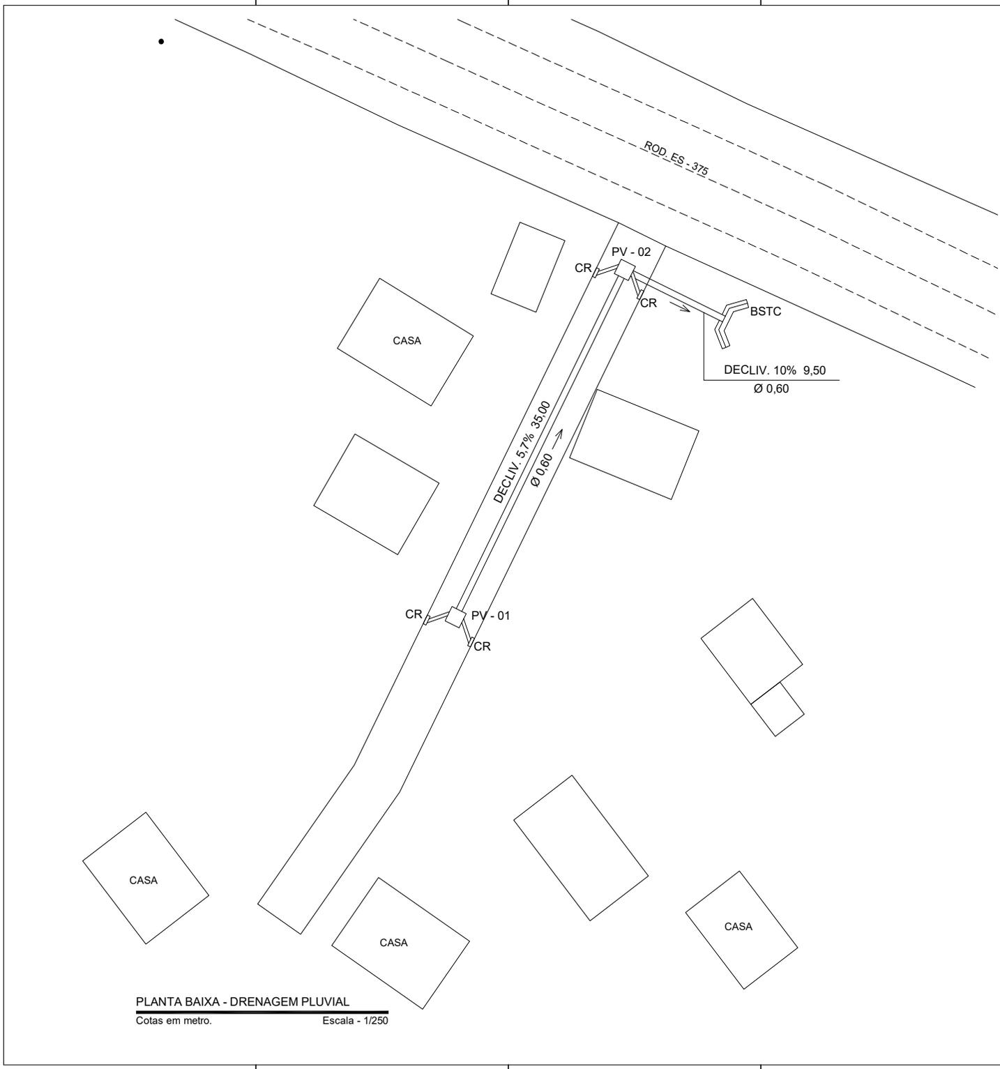
**PLANTA BAIXA - DRENAGEM PLUVIAL**
