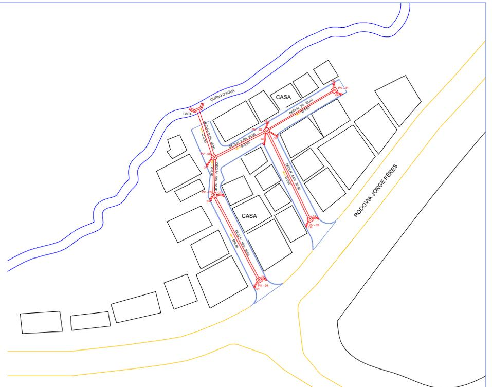
**PLANTA BAIXA - DRENAGEM PLUVIAL**
